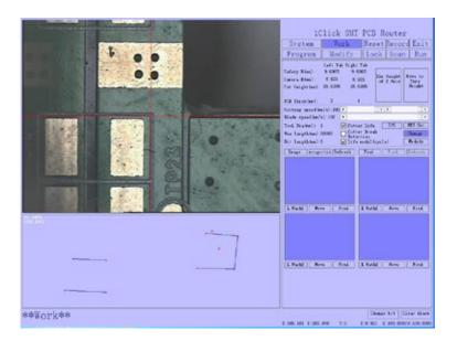
Milling cut can be used as 2 or 3 section , just set the parameter on sofeware , it has greatly prolonged milling cut' service life.
