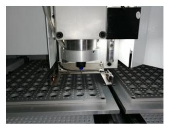
The machine is equipped with the broken milling cutter detection function on the spindle. When the milling cutter is broken, the machine will stop, and the software interface will alarm.
