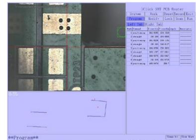
Self developed softeware makes programming and operating very easy .The software interface can set the Z-axis cutting depth and set different Z-axis cutting depths depending on the thickness of the PCB. Ensure that the Z-axis can cut the PCB at a fixed height (suitable for PCBs with components on the back of the cutting point, ensuring that the milling cutter does not damage the components on the back of the PCB).
